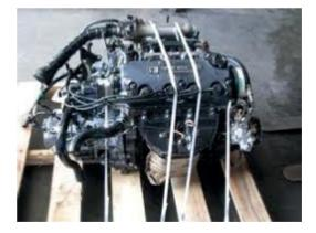
Plastic band strapped engine. 4 plastic straps done by machine and tight. Engine sits flat on pallet, no tyre needed. Ideally should be sat on rags/mat, but not needed as engine is drained, and is very clean. Straps could benefit from protection, but if bands touch smooth areas then are ok.
